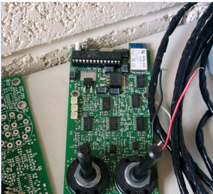
Fig. 13 The final board, with the RN-42 Bluetooth module.
