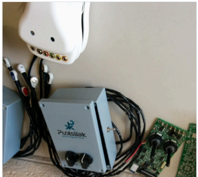
Fig. 14 The device with the Pulsilak brand and its electrode leads.
